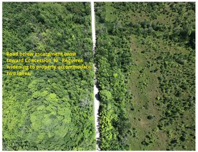
in road width, drainage and base structure which result in heavy maintenance and safety concerns. These maintenance requirements in turn have undesirable environmental impacts. These conditions, and impacts, are exacerbated by increasing levels of traffic which will only be accelerated by the pending closure of former County Road 91.
